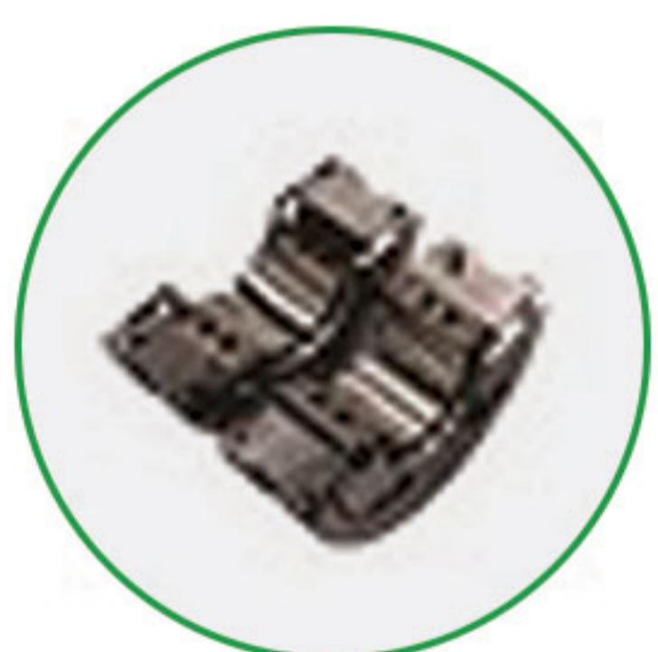
Tilting pad bearing can meet the vibration changing of Compressor with the ability of automatic alignment, the babbitt On the tile surface protects the shaft out of damage
