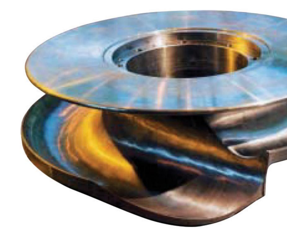
diaphragms perform the dual function of forming the diffuser passage (where gas velocity is transformed into pressure) and the return passage to channel gas to the eye of the next impeller. The discharge diaphragm forms the diffuser for the last impeller as well as the discharge volute. The diaphragms are usually horizontally-split.
